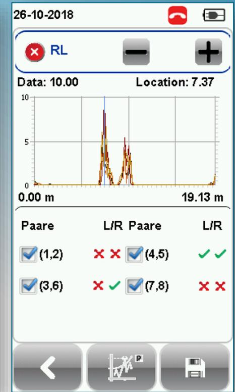
Return Loss failed because cable was run over and crushed by forklift truck after approx. 7m
